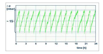
The pressure drop of the ALPHA Filter remains constant. The above plotting shows the performance characteristics with precoating and dP-controlled cyclic filter cleaning over a period of 24 hours. During the recording, the filter intake temperature was between 380 and 420° C.
